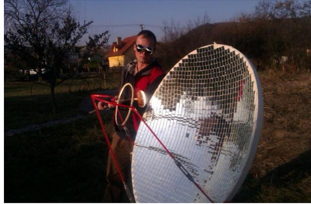
Solar collector from old parabola and mirrors
